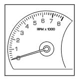
This gage indicates the engine speed in revolutions per minute (rpm).
